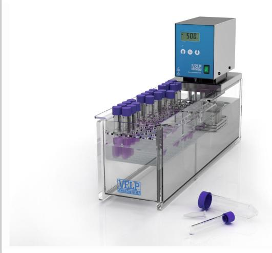
The open circulating bath is a widely used instrument, suitable for different applications and kinds of samples treatment. VELP OCB can reach 105 °C, with 1 °C steps, and can be combined with **different operating accessories** in order to satisfy any requirements and ensure reliable results.
